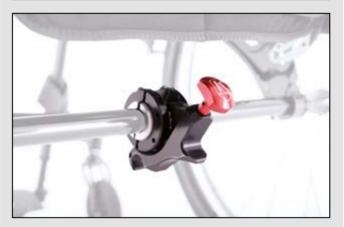
Rear Linking System Klaxon® for rigid wheelchair The system allows the Twist or Twist-R to be connected to the wheelchair in seconds, even by the user himself in manual or automatic mode (watch video). Its special configuration allows the wheelchair to be wheeled up, by the user or the caregiver, in order to overcome obstacles.
