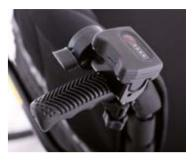
Releasing the accelerator lever, even accidentally, will instantly stop the motor thrust.
